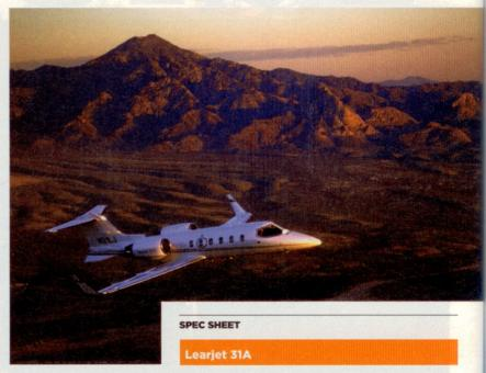
Engines | Two Honeywell TFE731-2-3B turbofans, 3,500 lbs thrust each Seats | up to 11 (including two crew)
